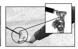
6. Attach ground wire (from step 5) to a ground rod (shown above), grounded fence wire or steel T post. Do not use the energizer's ground system.
