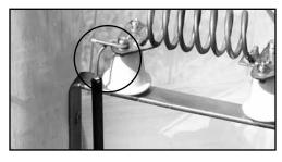
2. Attach an insulated lead wire from the energizer to either of the screws closest to the post.
