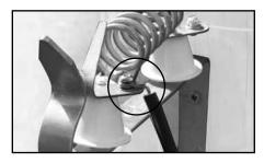
3. At the other end of the spring, connect an insulated wire using the provided screws.
